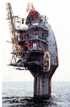
R/V FLIP (FLoating Instrument Platform), developed and still maintained by MPL for marine research, represents a novel approach to achieving more precise observations on board a vessel with its unique "flipping" design
